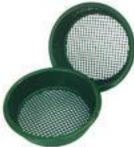
These sieves can range from extremely coarse devices that look like sewer grates for large size separations [range of inches] to sieves that look very much like window screens for middle separations [millimeter], to very fine woven screens for fine separations [~50 micrometers]. Separation can be either dry or wet. Wet screening is more efficient, but drying of the product adds cost.
